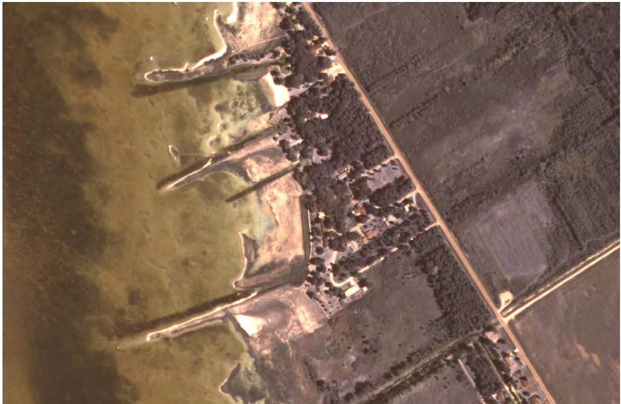
Figure 11. Airborne multispectral imagery (e.g., Positive System’s 1-meter spatial resolution, 4-band “ADAR” data) is available for specific areas and may be used to correlate land-use changes with wetland alterations, at local to regional scales, such as is shown in the Wildfowl Bay region of Saginaw Bay (Lake Huron).
