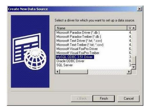
(v.) Next, the database links need to be defined. The default values are as shown below. The database name will need to be changed to the name of the particular folder which contains the MySQL database files (i.e., the MySQL database name).
