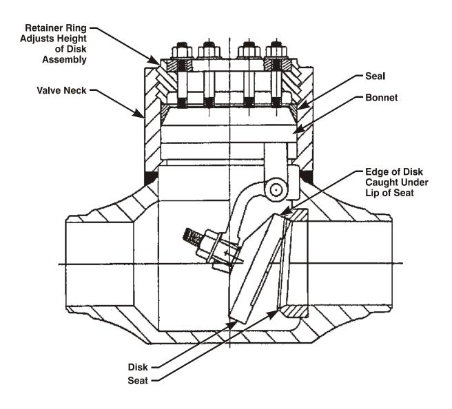
Figure 2. Borg-Warner Check Valve Shown with Disk Jammed in Open Position
