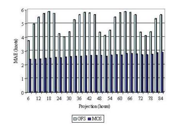
Figure 1. Overall mean absolute errors (MAE) in MOS and GFS wind speed forecasts, dry season, 0000 UTC, for 15 stations.
