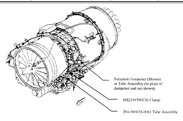
Figure 1. Hydraulic Tube Assembly with Clamp on Left Hand Engine.
