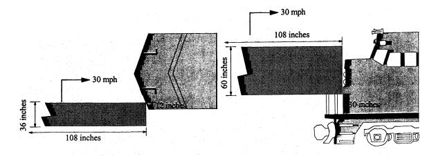
Figure 2. Schematic of Front End Structure (Short Hood) Offset Impact
