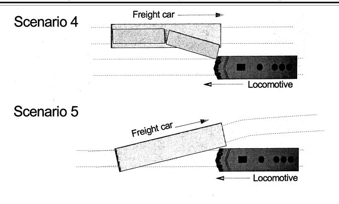
Figure 2. Schematics of Oblique Collision Scenarios.
