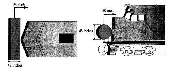
Figure 1. Schematic of Front End Structure (Collision Posts) Impact
