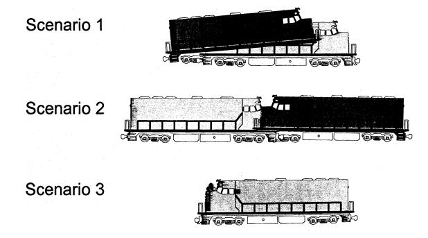
Figure 1. Schematics of In-Line Collision Scenarios.
