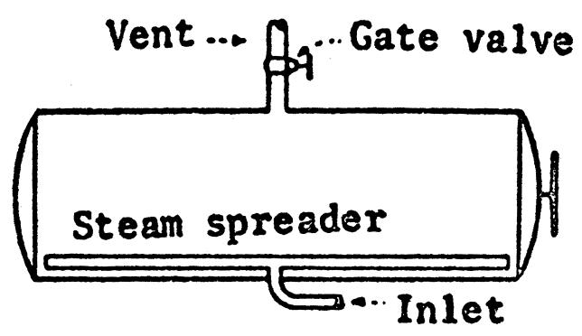
Specifications: A 2.5-inch (6.4 centimeters) vent equipped with a 2.5-inch (6.4 centimeters) gate or plug cock valve and located within 2 feet (61 centimeters) of the center of the retort.
