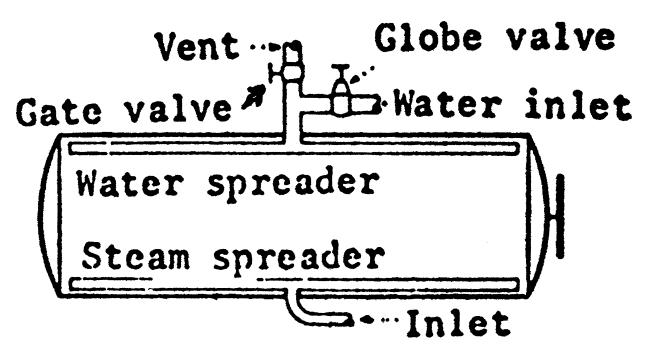
Size of vent and vent valve. For retorts less than 15 feet (4.6 meters) in length, 2 inches (5.1 centimeters); for retorts 15 feet (4.6 meters) and over in length, 2.5 inches (3.8 centimeters).
