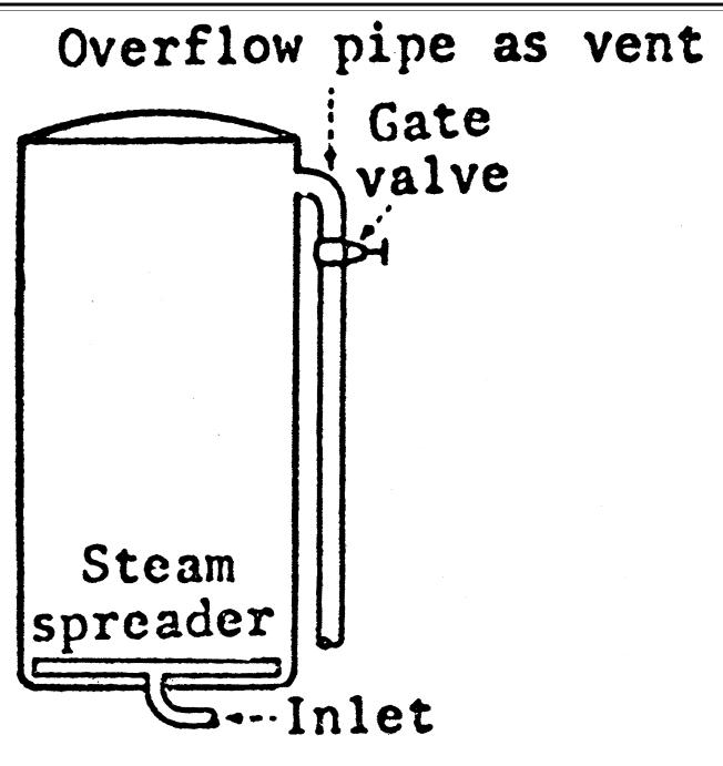
Specifications. A 1.5-inch (3.8 centimeters) overflow pipe equipped with a 1.5-inch (3.8 centimeters) gate or plug cock valve and with not more than 6 feet (1.8 meters) of 1.5-inch (3.8
