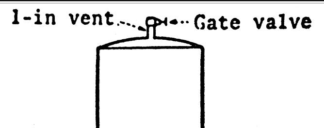
Specifications. A 1-inch (2.5 centimeters) vent in lid or top side, equipped with a 1-inch (2.5 centimeters) gate or plug cock valve and discharging directly into the atmosphere or to a manifold header.
