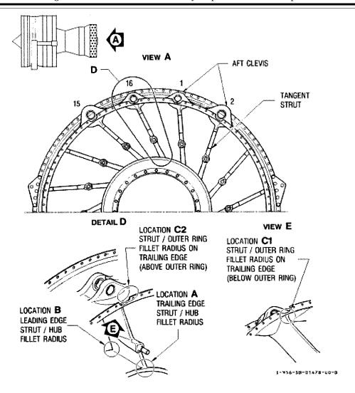
Turbine Rear Frame with Tangential struts P/N 340-166-205-0, 340-166-206-0, 340-166-207-0, 340-166-208-0, 340-166-209-0, 340-166-210-0—Areas to Be Inspected
