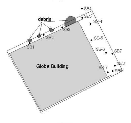
Figure 2 Locations of the soil boring (SB) and surficial soil (SS) samples on the Globe property in relation to the Globe building.
