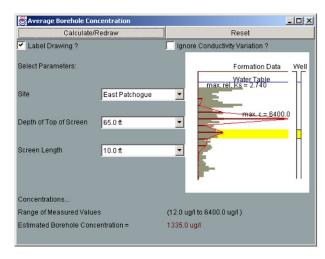
The Average Borehole Concentration calculator that is illustrating the concentration that would be seen in a well with a 10 foot long screen located 65 feet below the ground surface. The maximum peak concentration nearby this well was 6400 ug/l, but the effect of borehole averaging was to reduce the observed concentration to 1335 ug/l.
