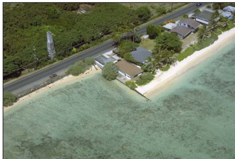
Many examples of natural beaches (right of groin) exist in stark contrast to narrow stretches of lost beach (left of groin) owing to shoreline harding (Kualoa, Oahu).
