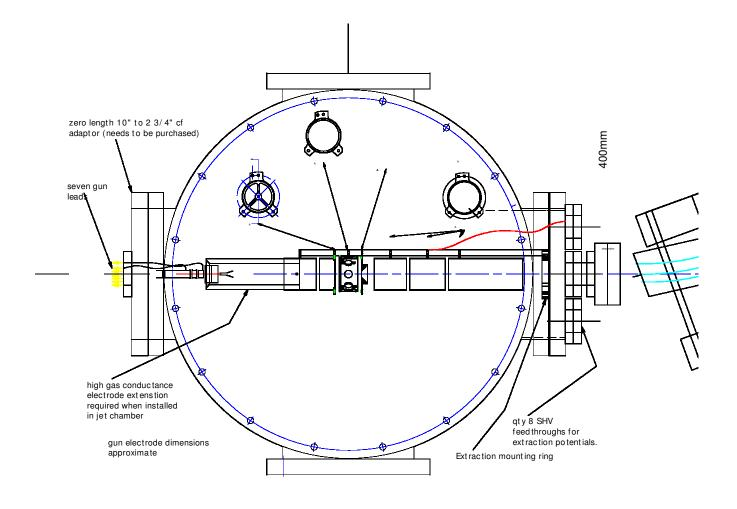
Electrons have same path as RHIC protons  $\Rightarrow$  measurement independent of beam profile
