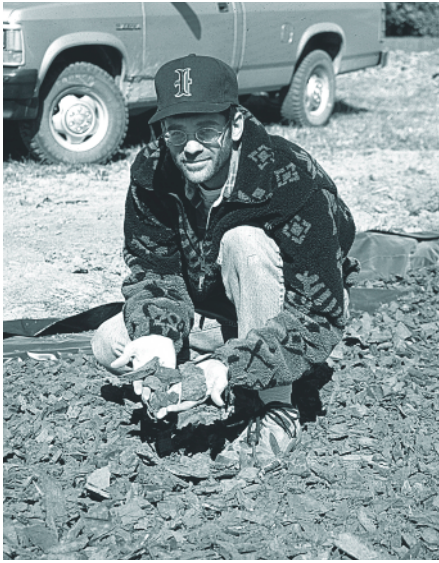
Tom Sperflage, Lake Fisher Watershed Project Coordinator, handles chipped tire used to upgrade 19 private household septic systems in the watershed.
