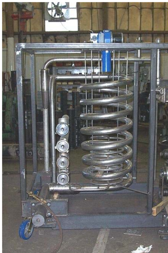
Figure 1. Gasifier under construction; the reactor coil (right) and four feed auger cylinders are shown.
