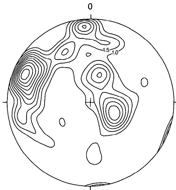
Lower-hemisphere, equal-area stereonet contour plot of probable relative orientation distribution density of fractures.
