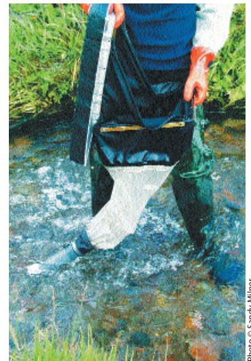
A Surber sampler is used to collect stream invertebrates
