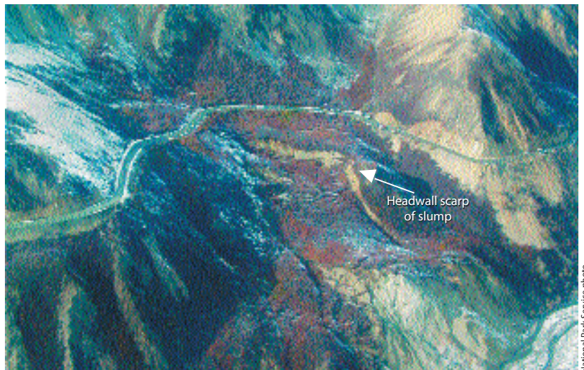
The landslide or slump at Milepost 45 threatens the park road
