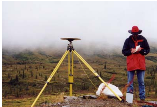
(b) 2002 Using GPS to measure movement near the Denali Fault (Photo credit: National Park Service, photo by Lucy Tyrrell)
