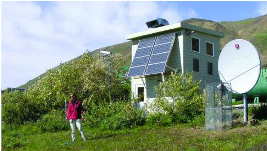
The Denali web camera, which runs on solar power, documents visibility conditions during the summer months. www2.nature.nps.gov/air/webcams/parks/denacam/denacam.cfm
