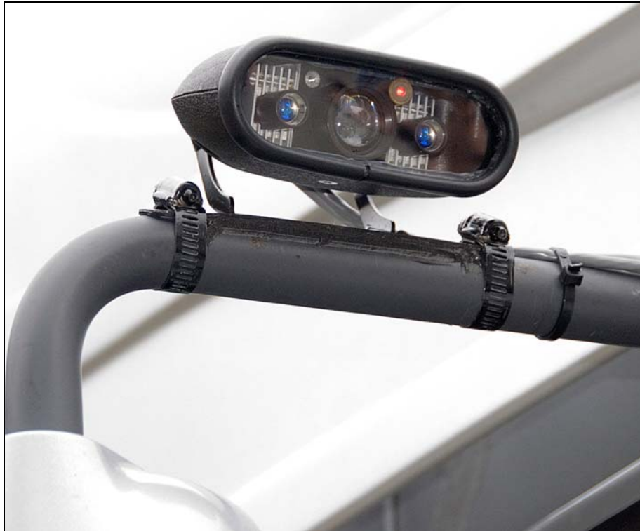
Figure 11. Road Surface Detection System Sensor
