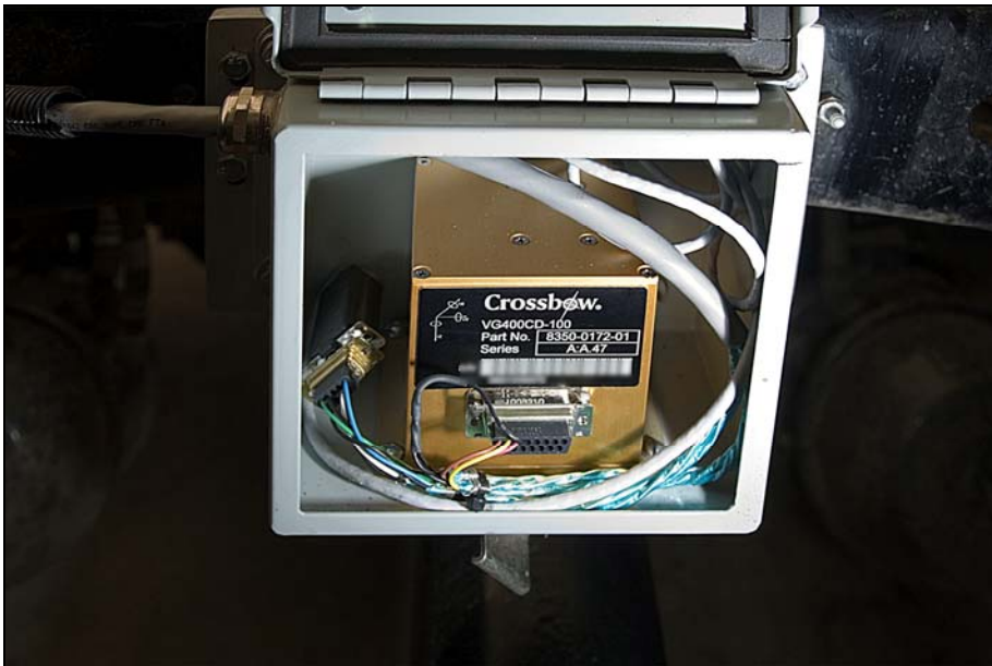
Figure 13. Rate Gyro and Accelerometer Enclosure (Opened)
