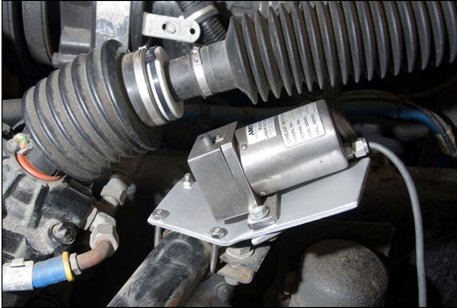
Figure 12. Steering Wheel Angle Sensor (String Potentiometer)
