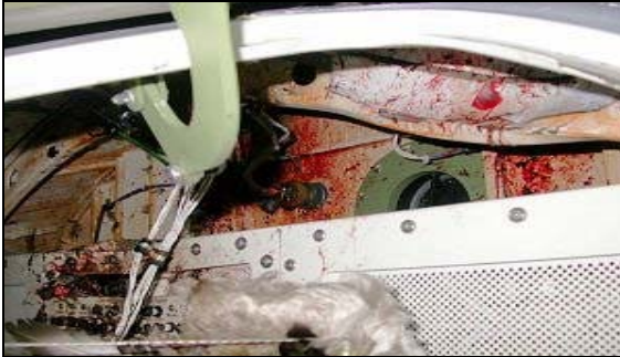
Pictured above - Bird-strike damage to an Nr 5 - Horizon DHC-8. It occurred in Medford, Oregon, on January 8, 2003.
