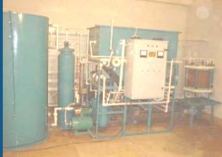
The "Dial-5" desalinating device with productivity of 0.3 to 1.0 m 3 /h.
