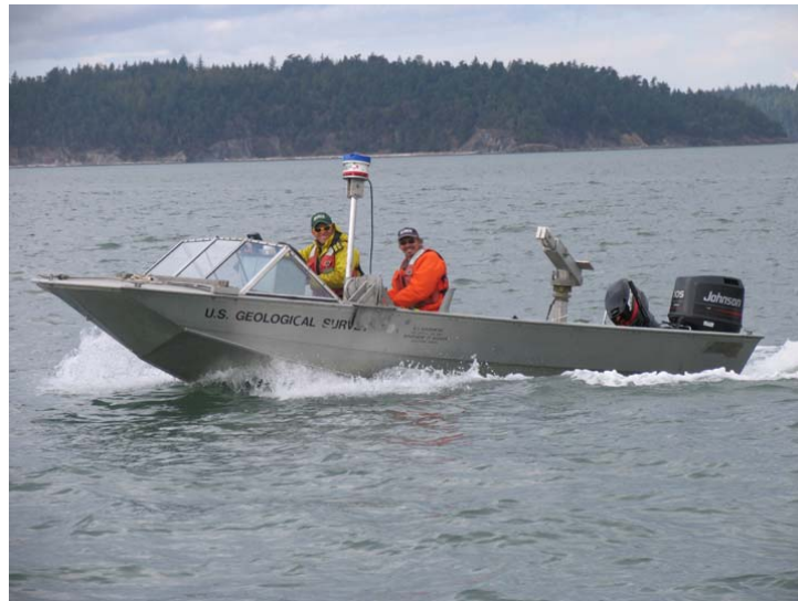
Figure 7. Photograph of the roving Acoustic Doppler Current Profiler and Differential Geographic Positioning System setup.
