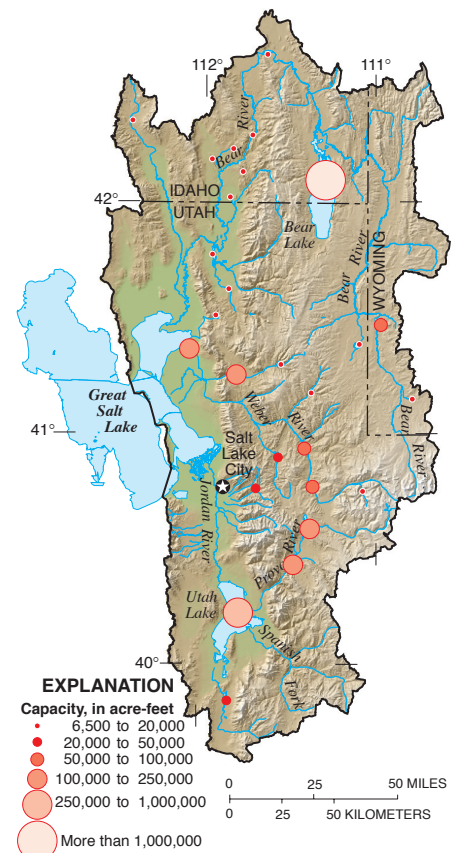
Figure 4. Reservoir capacity in the Great Salt Lake Basins Study Unit exceeds 3.5 million acre-feet.
