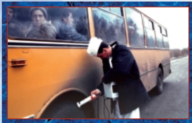
A worker checks departing automobiles for radiation levels near the TOMSK-7 plutonium processing facility in Russia.
