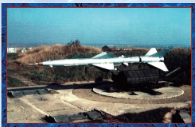
Side view of Hungarian SA-2 Guideline mounted on a fixed launcher.
