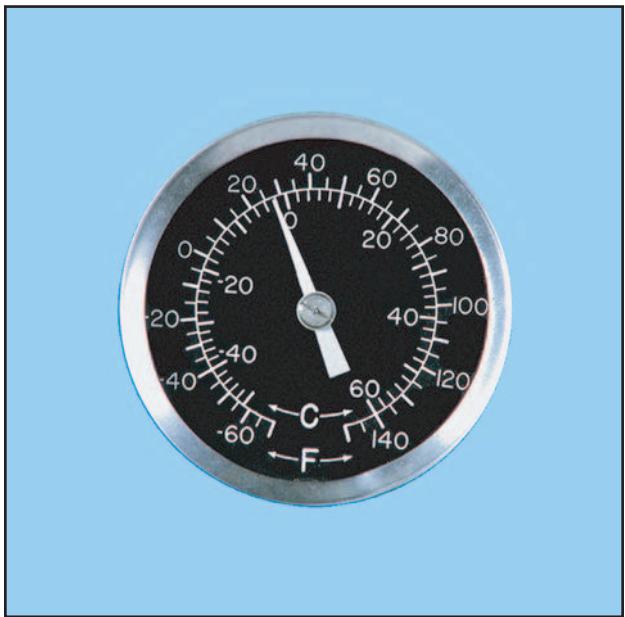
Figure 6-24. Outside air temperature gauge.
