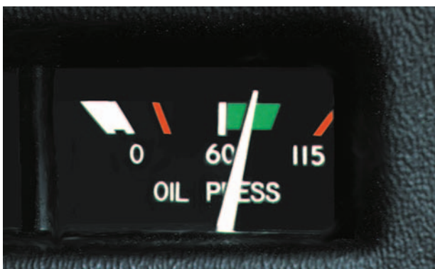
Figure 7-3. Minimum, maximum, and normal operating range markings on oil gauge.
