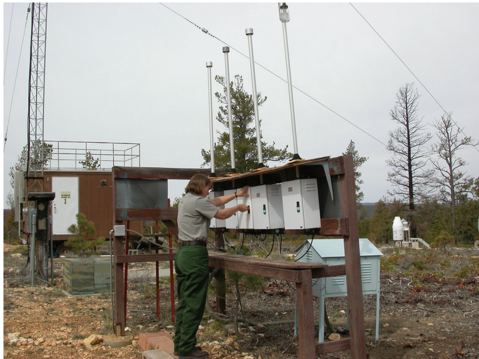
Air-quality monitoring station at Bryce Canyon National Park, Garfield County, Utah. Photograph by Mark Miller, USGS.
