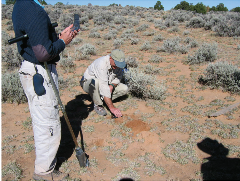
USGS geologist measuring soil magnetic properties to support studies relating vegetation patterns to geomorphic processes affected by climate and land use. San Juan County, Utah. Photograph by Mark Miller, USGS.
