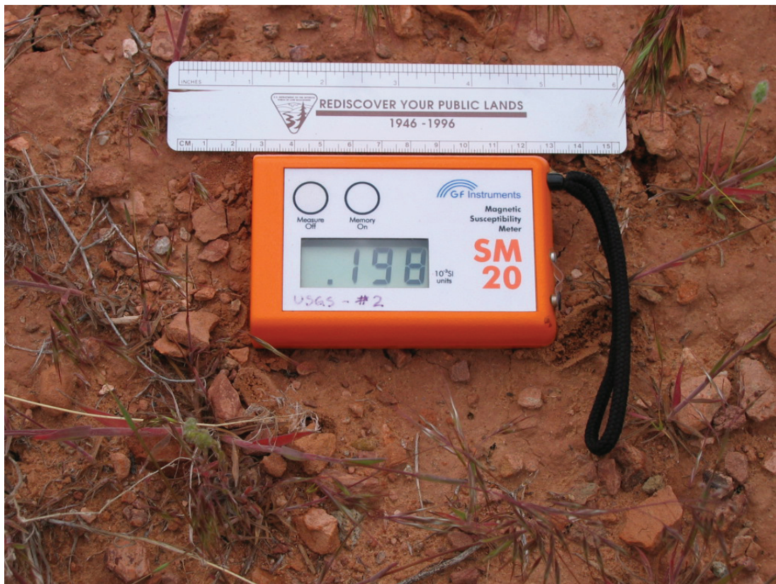
Magnetic susceptibility meter used for measuring magnetic properties of soils and rocks. San Juan County, Utah. Photograph by Mark Miller, USGS.
