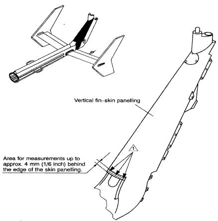
riangle Measurements are to be taken at at least three locations on the skin panel of the vertical fin. Care has to be taken that the external calipers are held squarely to the skin panel wall while measurements are being taken, since tilting of the calipers can lead to false results. If the panel thickness, including the primer coating, is at least 0.778 mm (0.03063 inch) at every measured location, no further action is necessary.
