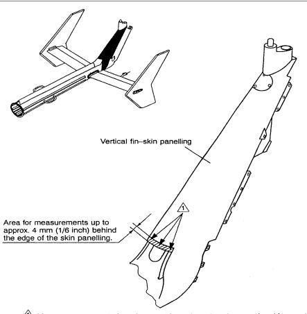
A Measurements are to be taken at at least three locations on the skin panel of the vertical fin. Care has to be taken that the external calipers are held squarely to the skin panel wall while measurements are being taken, since tilting of the calipers can lead to false results. If the panel thickness, including the primer coating, is at least 0.778 mm (0.03063 inch) at every measured location, no further action is necessary.
