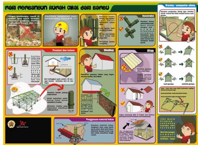
A USAID-funded poster in Indonesia that shows how to create seismically resistant bamboo structures.
