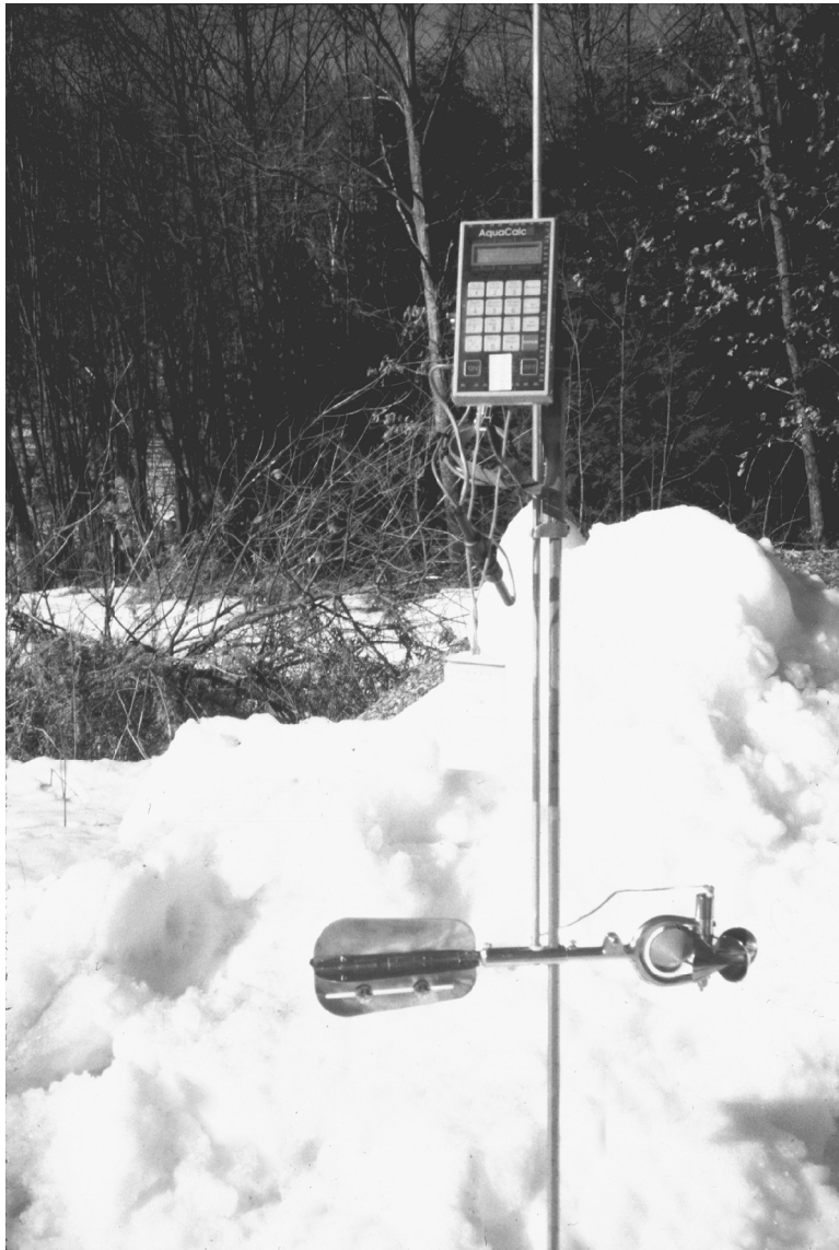
Primary tools of USGS streamgaging; top-setting wading rod, rotating-bucket current meter, and discharge measurement computer. (photo by J.L. Zanca)
