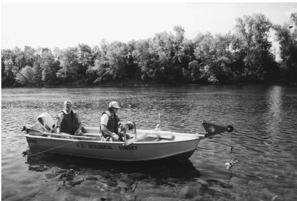
Streamflow discharge measurement by boat, Connecticut River at Montague City, Mass., Aug. 16, 1995 (photo by R. S. Socolow).
