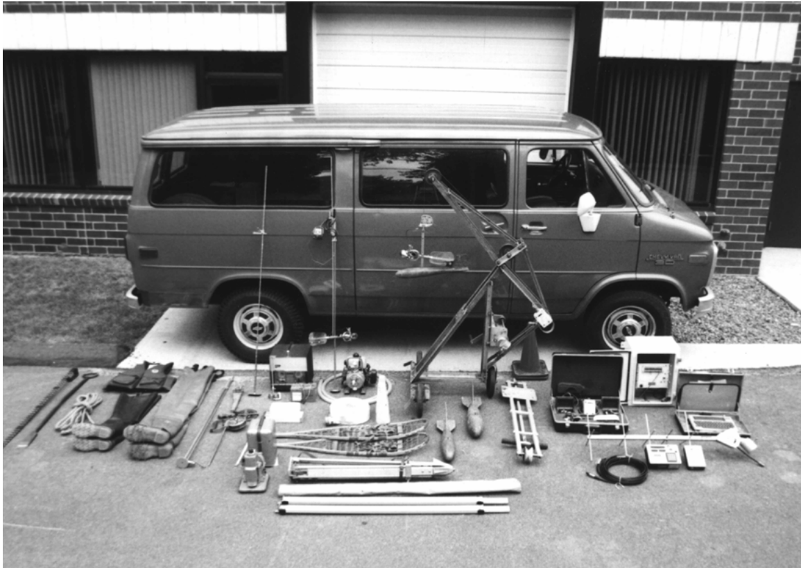
Typical complement of streamgaging equipment carried in USGS field vehicles (photo by R. S. Socolow).
