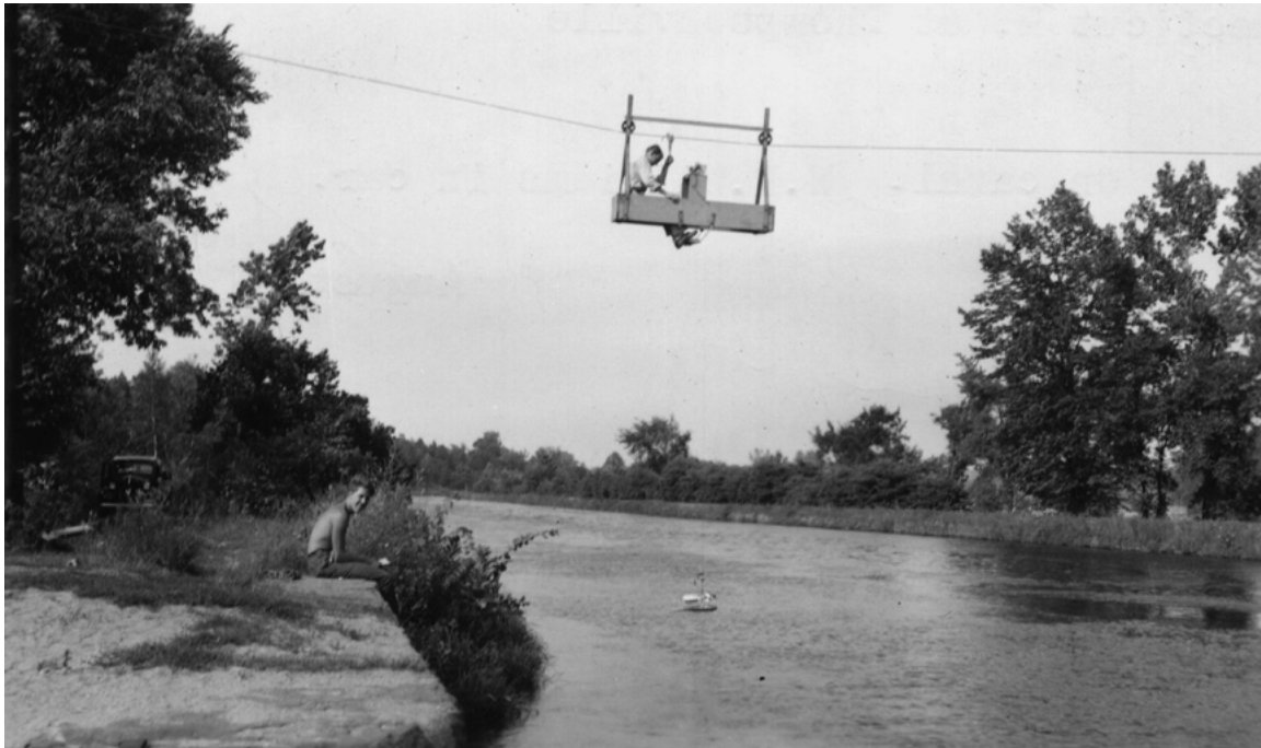
Streamflow discharge measurement by cable-car on diversion canal, Connecticut River at Thompsonville, Conn., 1939.
