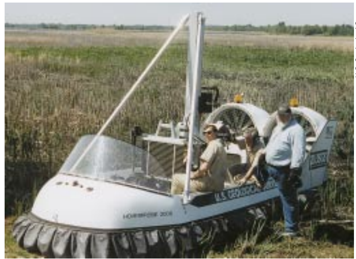
Figure 4. Hoverprobe drilling in an area not accessible by boats or trucks.
