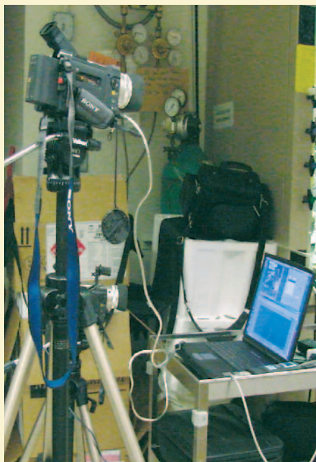
Focused on health. Detectors (above, in backpack) collect real-time exposure data, which are sent to a computer (left) and merged with footage of the worker performing a procedure. The result is a video “diary” showing fluctuations in exposure corresponding with each step in the procedure.
