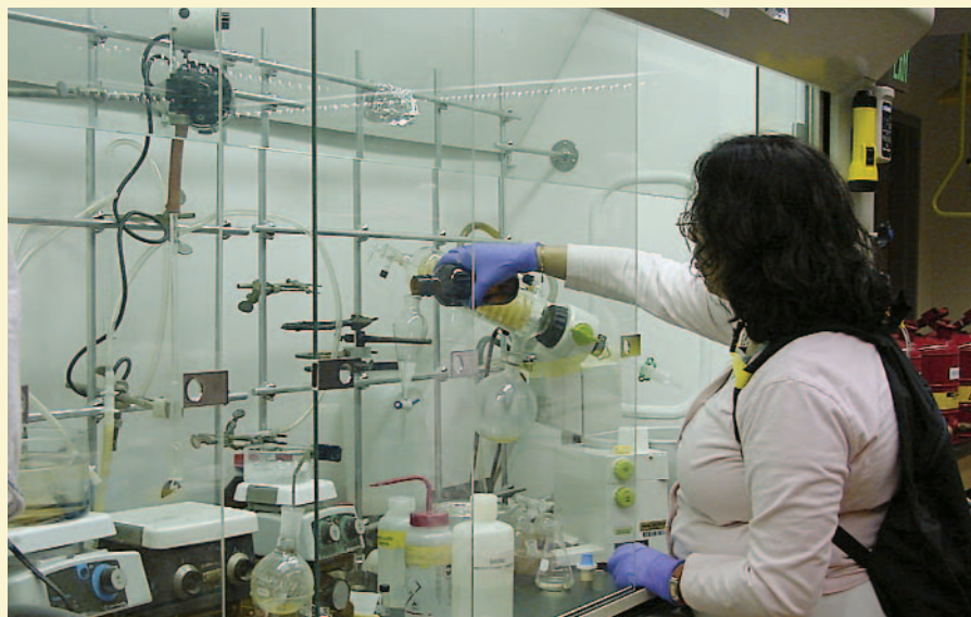
Focused on health. Detectors (above, in backpack) collect real-time exposure data, which are sent to a computer (left) and merged with footage of the worker performing a procedure. The result is a video “diary” showing fluctuations in exposure corresponding with each step in the procedure.
