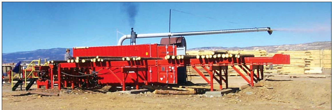
Figure 2—SLP5000 Diesel Micromill ® processing small-diameter ponderosa pine (Photo by Dean Parry).
