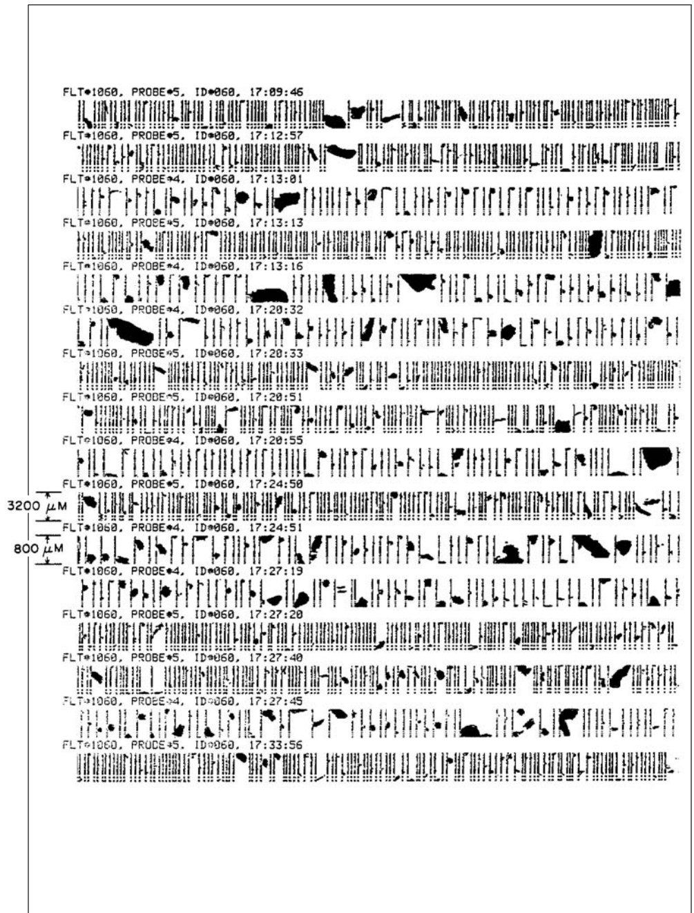
Figure 21—Shadow images of airborne particles observed with the laser camera in cross-sectional sequence 2 through the plume from the burn, ≈1727 PDT, September 15, 1982. For probe 4, the vertical frame size is 800 μm; for probe 5, it is 3200 μm.
