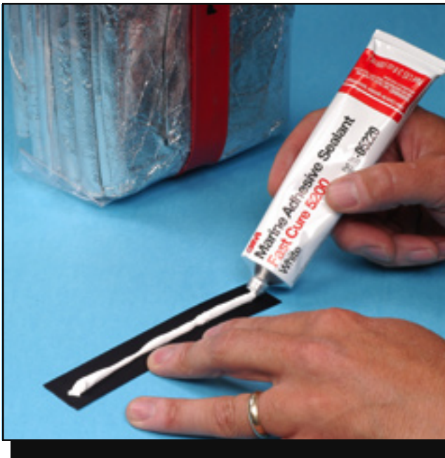
STEP 1: Apply a thin bead of adhesive to the nylon webbing.
