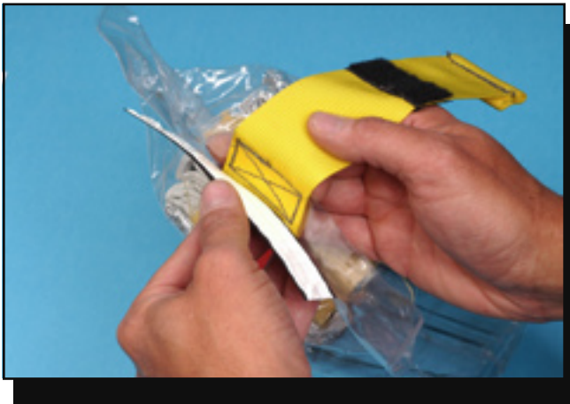
STEP 3: Apply the webbing to one side of the pull strap attachment area and smooth it in place. Repeat on the opposite side of the pull-strap attachment area.
