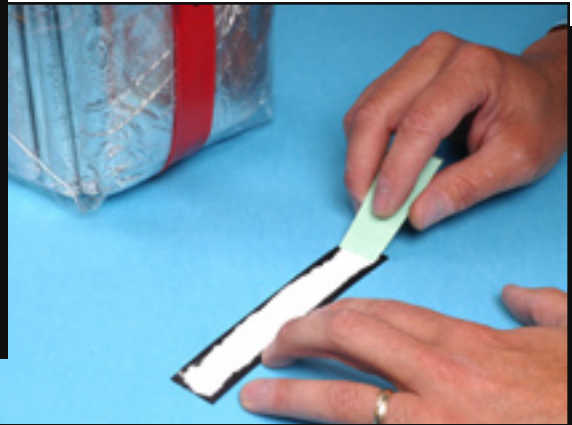
STEP 2: Spread adhesive so it is \frac{1}{16} inch thick.
