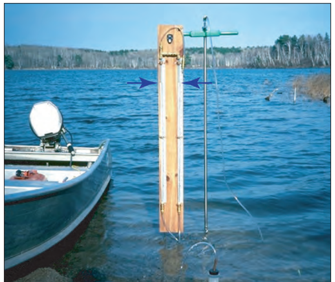
Figure 5. Hydraulic potentiomanometer showing drive probe inserted into lakebed and manometer indicating a very small vertical hydraulic-head gradient (blue arrows indicate water levels on manometer). (Photograph by Donald Rosenberry, U.S. Geological Survey.)
