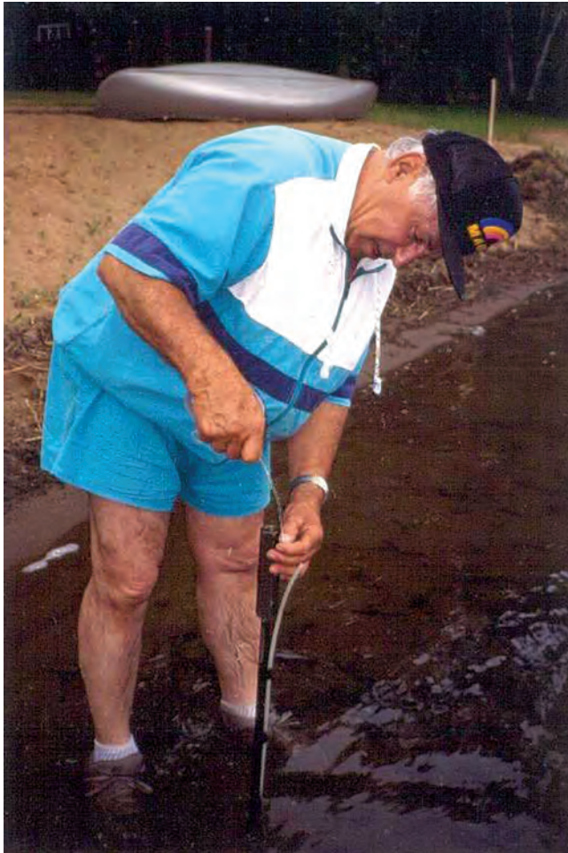
Figure 10. Portable well probe consisting of a commercially available retractable soil-gas vapor probe connected to threaded pipe with tubing inside the pipe connected to the vapor probe. A separate tube taped to the outside of the pipe extends to the lake-water surface. (Photograph by Donald Rosenberry, U.S. Geological Survey.)
