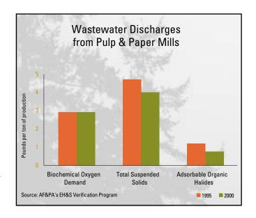
In compliance with EPA's Pulp and Paper Cluster Rule, which requires the reduction of toxic pollutants released to water and air, the industry has substituted chlorine dioxide for elemental chlorine as a bleaching agent, virtually eliminating dioxin from its wastewater. This substitution has also resulted in a 37% reduction of AOX, which is an indicator of chlorinated organic substances, between 1995 and 2000.<sup>19</sup>
