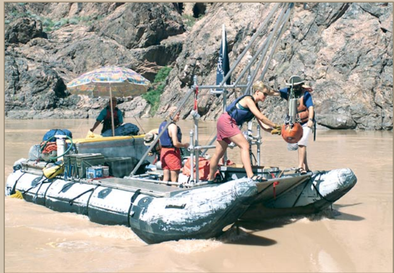
U. S. Geological Survey raft deploying underwater microscope system in the Colorado River.
