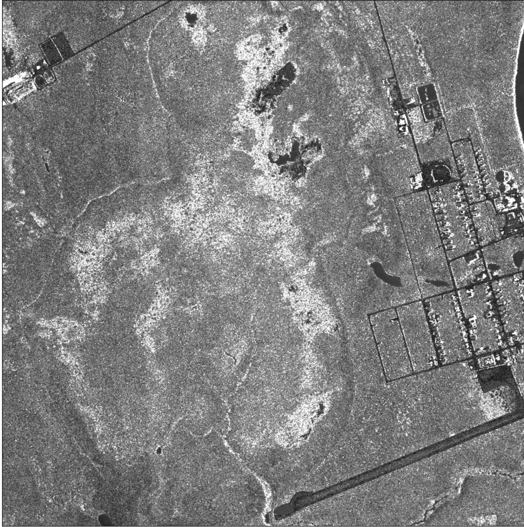
Figure 1. ORRI of Nuiqsut area, North Slope, Alaska. Although ORRIs resemble grayscale aerial photographs, each pixel value actually represents the magnitude of sensor signal return.
