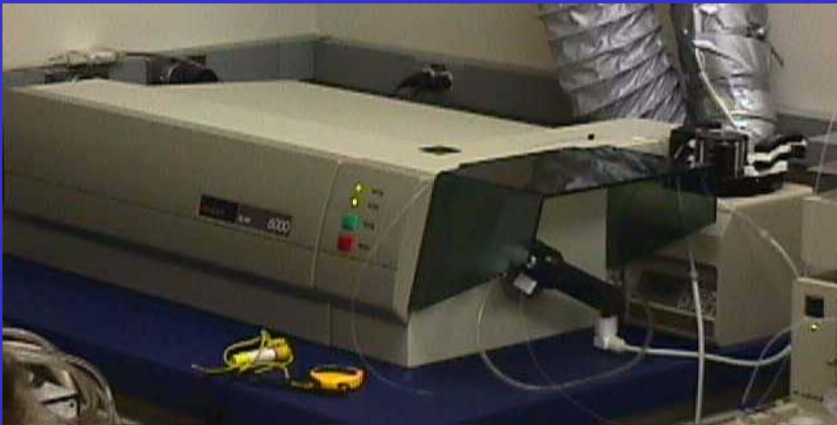
Figure 17. Photograph showing equipment used for dissolved-metal analysis by inductively coupled plasma mass spectrometry (ICP-MS)
