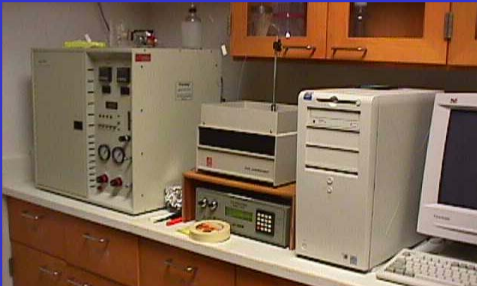
Figure 16. Photograph showing equipment used for dissolved organic carbon (DOC) analysis by high-temperature, non-catalytic oxidation.
