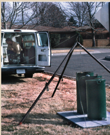
A USGS hydrologist using geophysical-logging equipment at the Del Sol Divider monitoring well.
