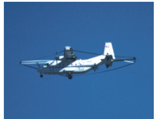
A converted Spanish transport plane used for airborne time-domain electromagnetic surveys in the Middle Rio Grande Basin. The wires wrapped around the plane compose the transmitting antenna.
