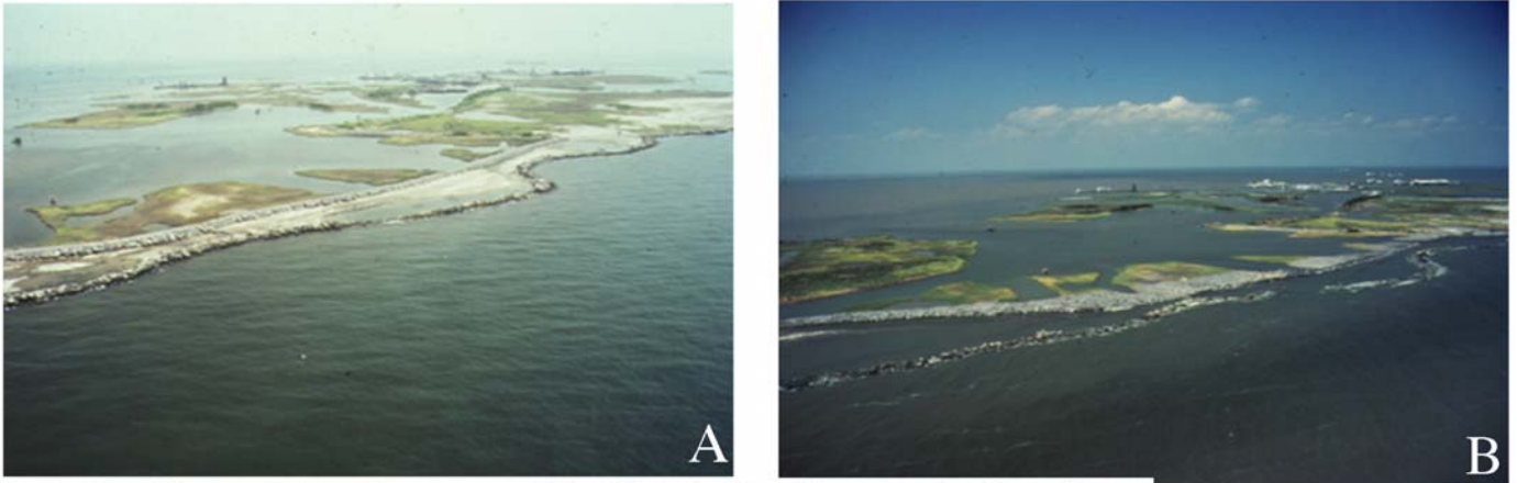
Figure 6. Photographs taken 7 weeks apart of East Timbalier Island illustrating the effects of Hurricane Andrew along this armored, low-sediment shoreline. Loose sand was removed and the rocks of the seawall were rearranged: A) Before - taken July 9, 1992, and B) After - taken August 30, 1992.
