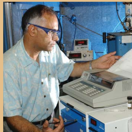
Devinder Mahajan uses a gas chromatograph to analyze carbon monoxide levels in hydrogen purified using his patented process.
