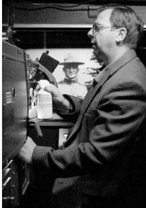
Ed Autry, an audiovisual technician at the Harry S. Truman Library in Independence, MO, uses compressed air to clear debris from the film gate of a 35mm projector. (Photo by Jamie Oakes)
