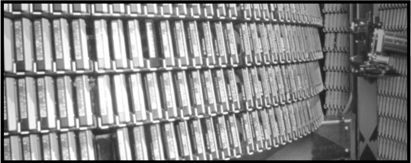
The robotic arm and shelves of tapes inside one of the five StorageTek 9310 tape silos at the San Diego Supercomputer Center, where much of our ERA research is being done. (Photo courtesy, SDSC)
