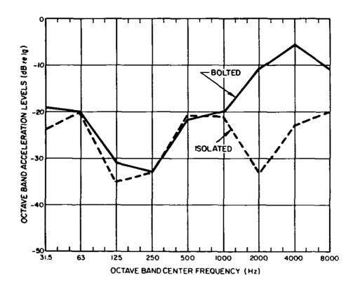
Figure 6.3.1. Vertical acceleration on pier, before and after isolation.
