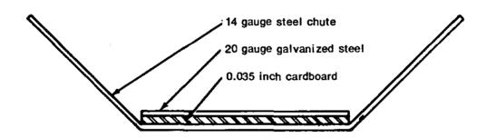
Figure 6.6.1. Chute for conveying cartridge cases.
