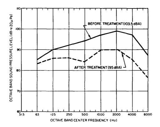
Figure 6.4.1. Operator position sound pressure levels, before and after treatment of nail-making machine.
