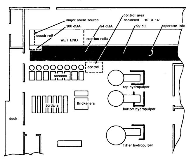
Figure 6.1.1. Paper mill - wet end.
