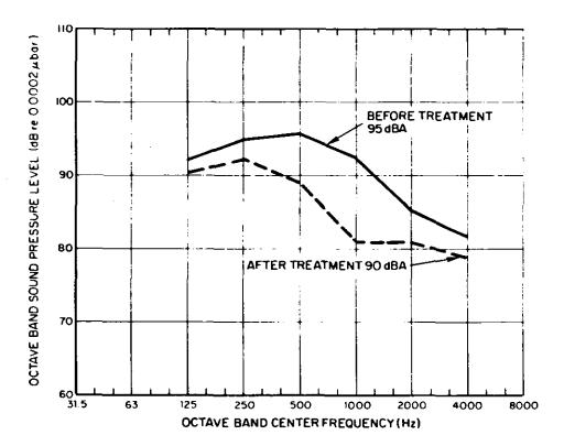
Figure 6.2.1. Reduced aisle sound levels, as predicted.
