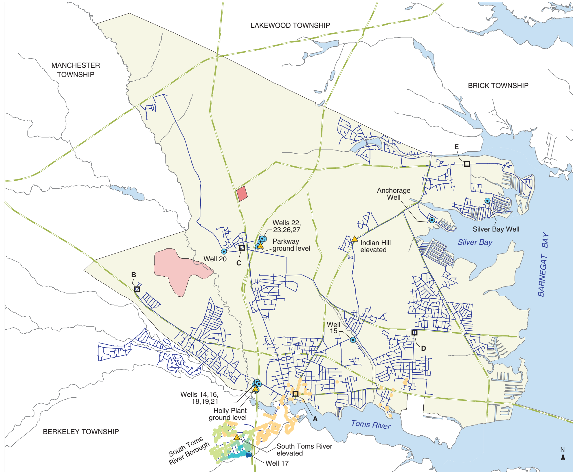
PLATE 79. AREAL DISTRIBUTION OF SIMULATED PROPORTIONATE CONTRIBUTION OF WATER FROM THE SOUTH TOMS RIVER WELL (17) TO LOCATIONS IN THE DOVER TOWNSHIP AREA, NEW JERSEY, OCTOBER 1971 CONDITIONS
