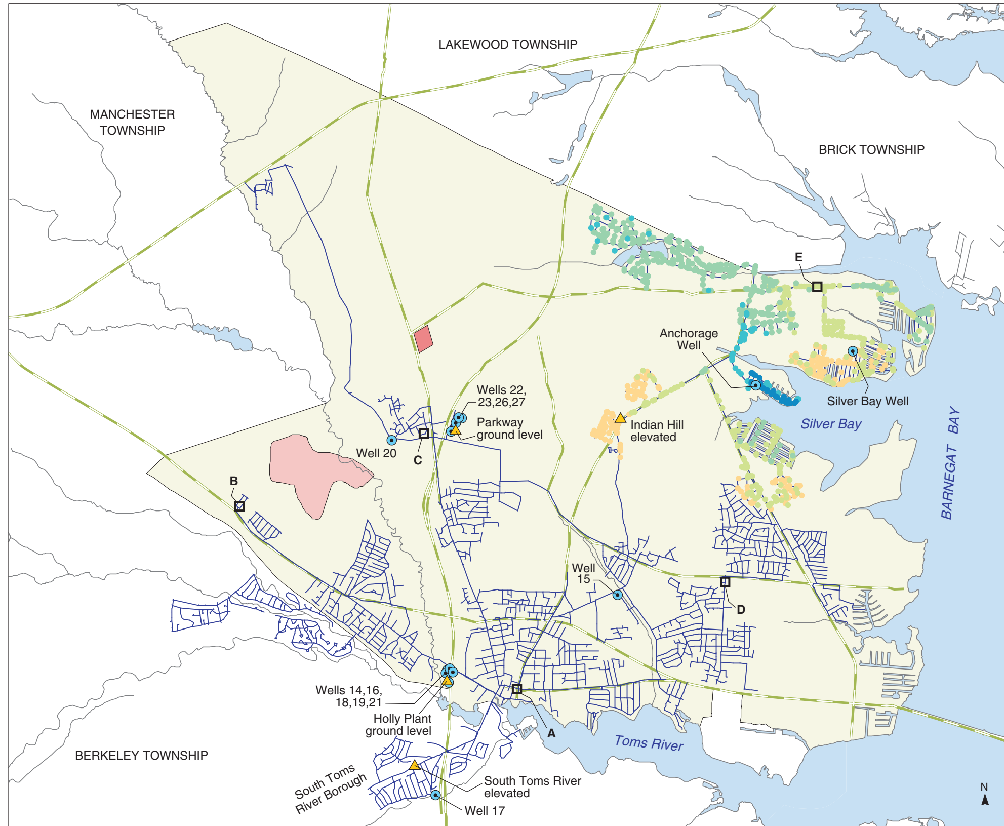
PLATE 75. AREAL DISTRIBUTION OF SIMULATED PROPORTIONATE CONTRIBUTION OF WATER FROM THE ANCHORAGE WELL TO LOCATIONS IN THE DOVER TOWNSHIP AREA, NEW JERSEY, JULY 1971 CONDITIONS
