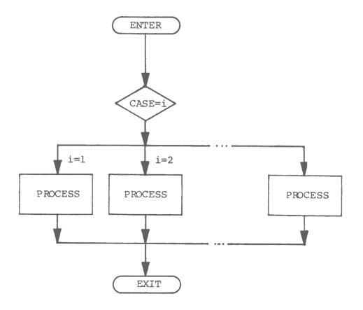
Control is passed to a Process based on the value of i.
