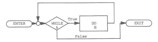
Condition "A" is evaluated. If found to be true, then control is passed to Process "B" and condition "A" is reevaluated. If condition "A" is found to be false, then control is passed out of the loop.
