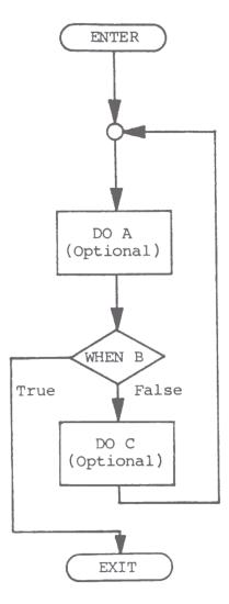
Optional process A is executed. Condition B is then evaluated. If found to be false, optional process C is executed and control is passed to process A. Condition B is then evaluated again. If condition B is true, then control is passed out of the loop.
