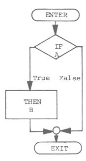
*Option* - Flow of control will skip a process pending the condition of "A."
