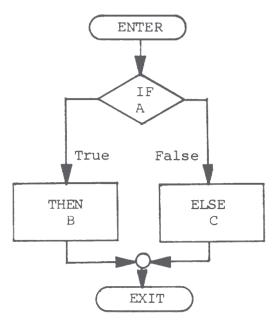
**Basic** - Flow of control will return to common point after executing Process "B" or "C". "A" predicates the conditional execution.
